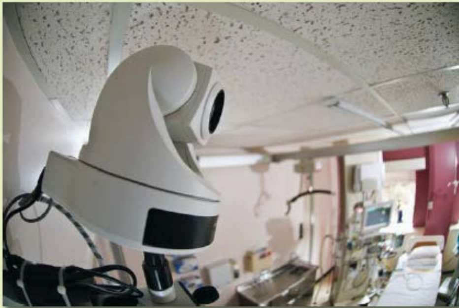
Figure 1 High-resolution cameras with zoom and pan ability are mounted in each room in the intensive care unit, enabling the tele-ICU staff to assess patients and/or communicate directly with the bedside team.
